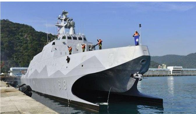
*A high efficiency wave-piercing catamaran hull form was selected for its greater stability and shallower draft characteristics. (Lung Teh)*
