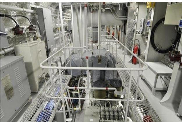
*The engineering space in Tuo Jiang. The ship is outfitted with four MJP CSU 850 water-jet propulsion systems that enable it to achieve a maximum stated speed of 43 kt. (Lung Teh)*
