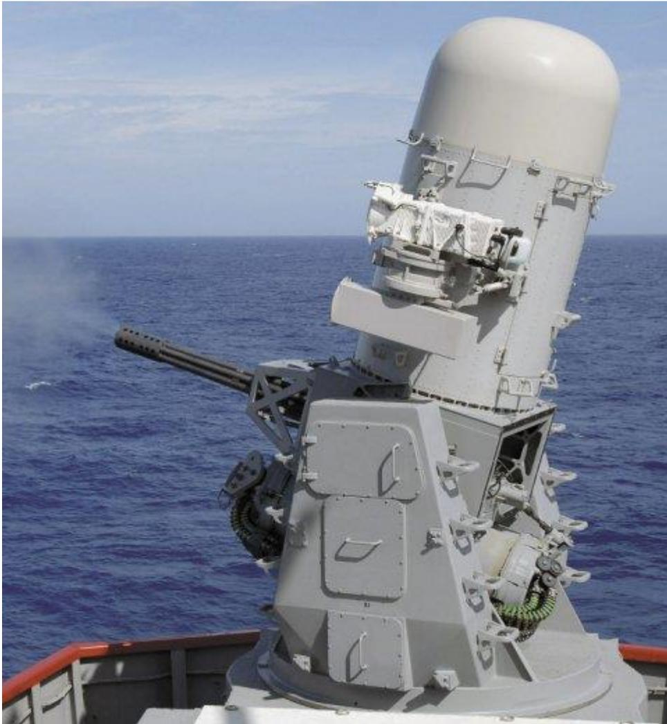
*The Block 1B upgrade package adds a surface engagement mode for the Phalanx CIWS. (US Navy)*
